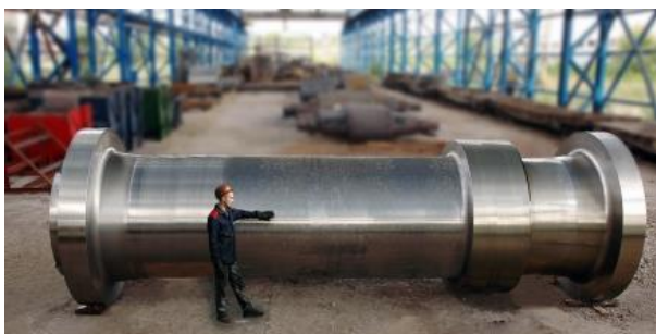
Figure 3 Turbine power shaft with weight of 220 tons after machining
