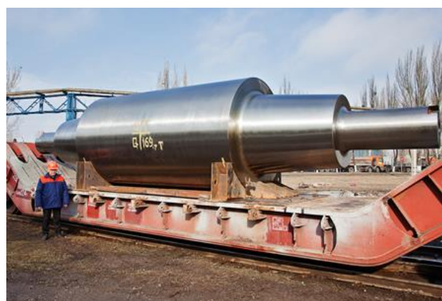
Figure 2 The backup roll weight of 165 tons after machining
